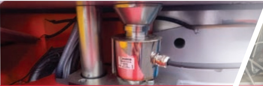
01 Weighing sensors to control the cakes release system and calculation of the cakes dryness
